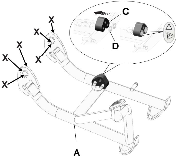
**GB** Lubricate the points (X) as shown in the figure with water-resistant grease.
